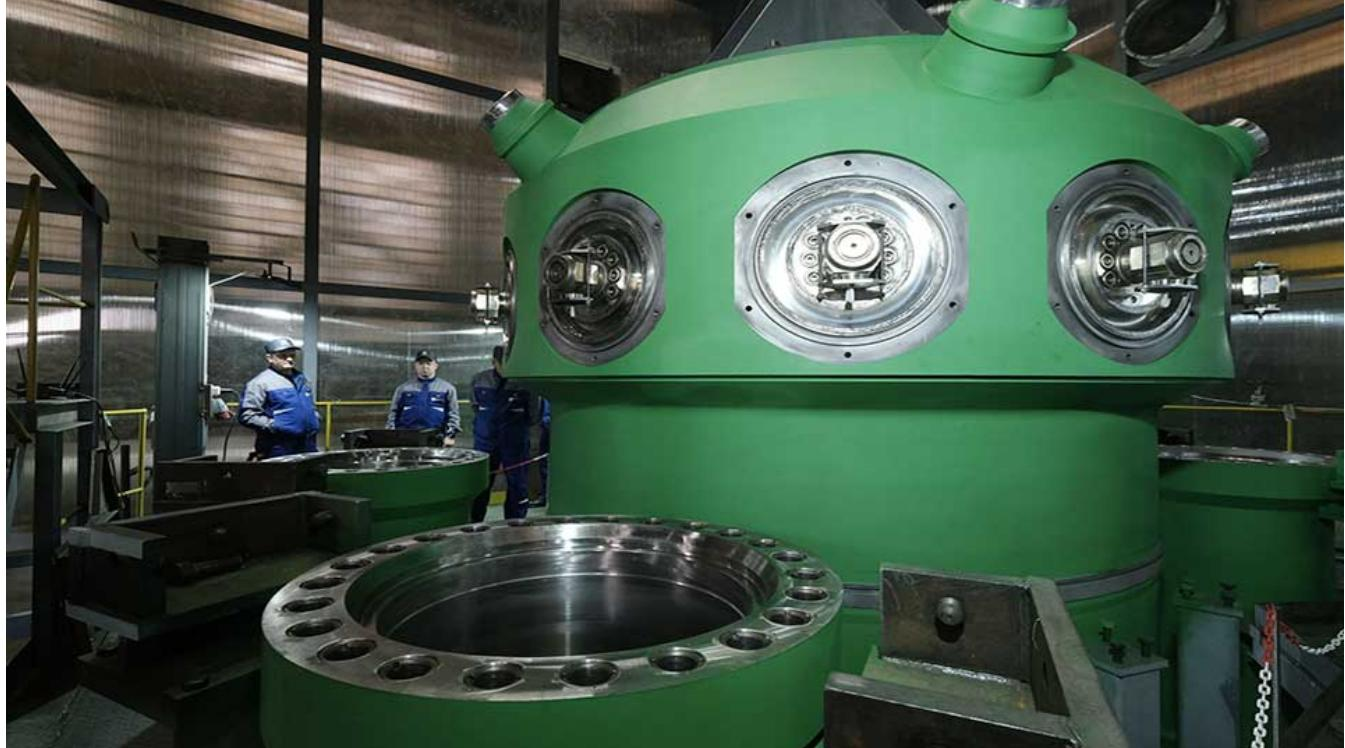
**Manufacturing of the first RITM-400 reactor, the most powerful in the world, has been completed by Rosatom. The reactor will be used in the nuclear icebreaker Rossiya. The icebreaker will have two such reactors.**
