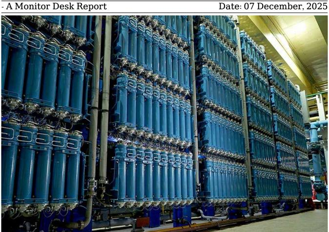
The first block of high-performance 9+ generation gas centrifuges has been launched at the Isotope Separation Plant of the Siberian Chemical Combine in Seversk, Russia. The plant is an enterprise of Rosatom's Nuclear Fuel Division. The Isotope Separation Plant at the Siberian Chemical Combine is the third of Rosatom's four enterprises engaged in uranium enrichment to introduce gen. 9+ centrifuges.
